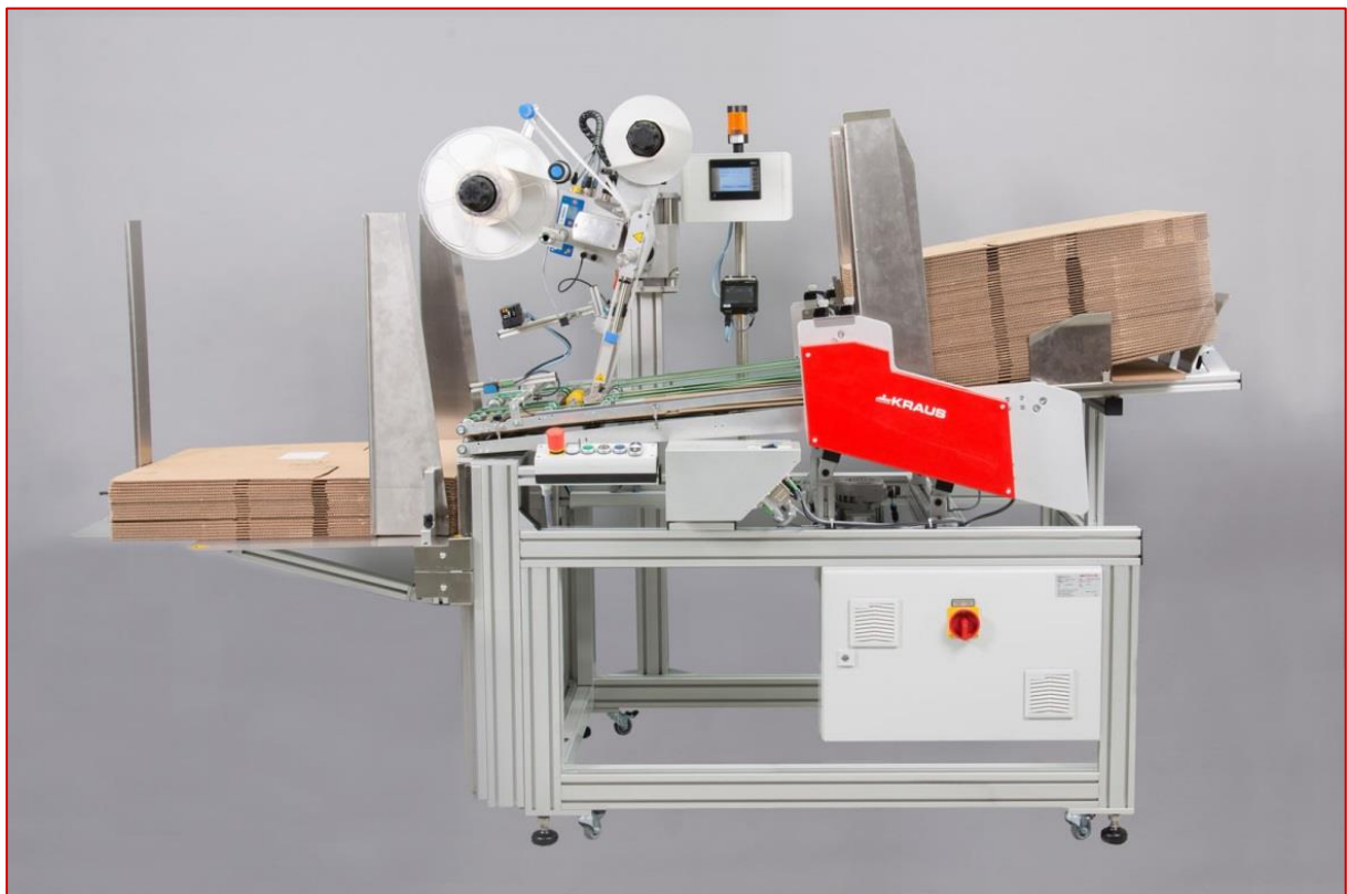
Integrated labelling system in the friction feeder's discharge extension
