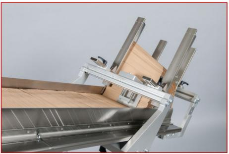
Vertical magazine chute on the shingle feeding belt with retention mimic for perfect shingling of the products on the belt.
